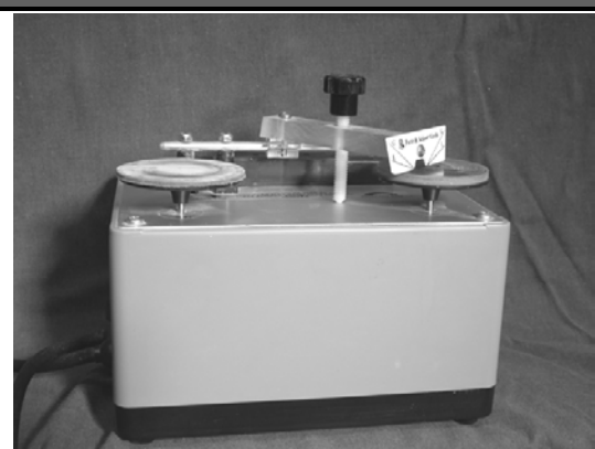
Figure #9.15. The Rx Honing Machine. It comes with a diamond wheel for rapid grinding, a carbide composite wheel for fine sharpening and a leather strop wheel for a polished finish. There are also a variety of reciprocating stones that attach to the far side of the machine for a variety other sharpening functions. The sharpening guide hovering over the wheel on the right is used to align scaler, curettes and scissors at the proper angle for sharpening.
