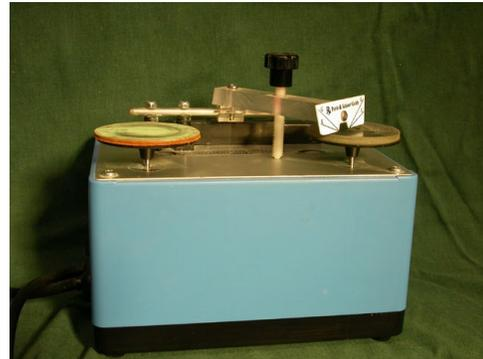
Hand Instruments should be sharpened after every use. While this can be achieved with hand-operated stones, a sharpening machine like the Rx Honing System (<http://www.rxhoning.com>) is going to be a good investment. This can be obtained from Dentalaire and/or BorderLink (and possibly other distributors as well).
